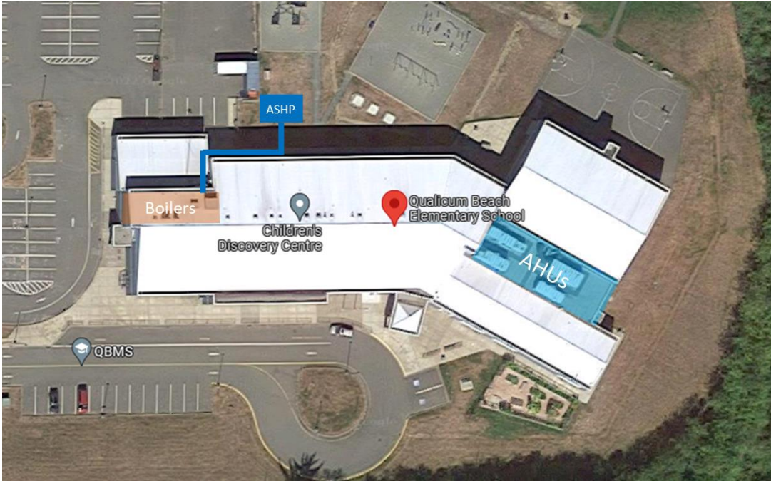
Figure 22: Possible alternative locations for an air-source heat pump connected to the heating loop
